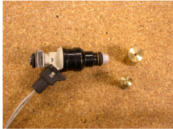
Figure 6 Image of three types of pressure simplex atomizers examined in this study. The larger, solenoid controlled nozzle is an automotive spray injector.
